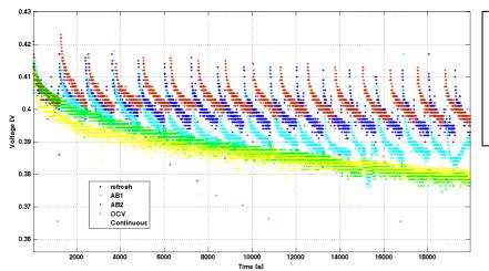
DMFC single cell operation at Polimi → Refresh cycles applied to reduce reversible performance degradation
