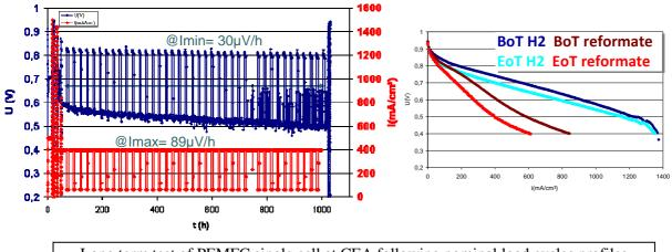
Long term test of PEMFC single cell at CEA following nominal load cycles profiles under critical fuel composition conditions condition
